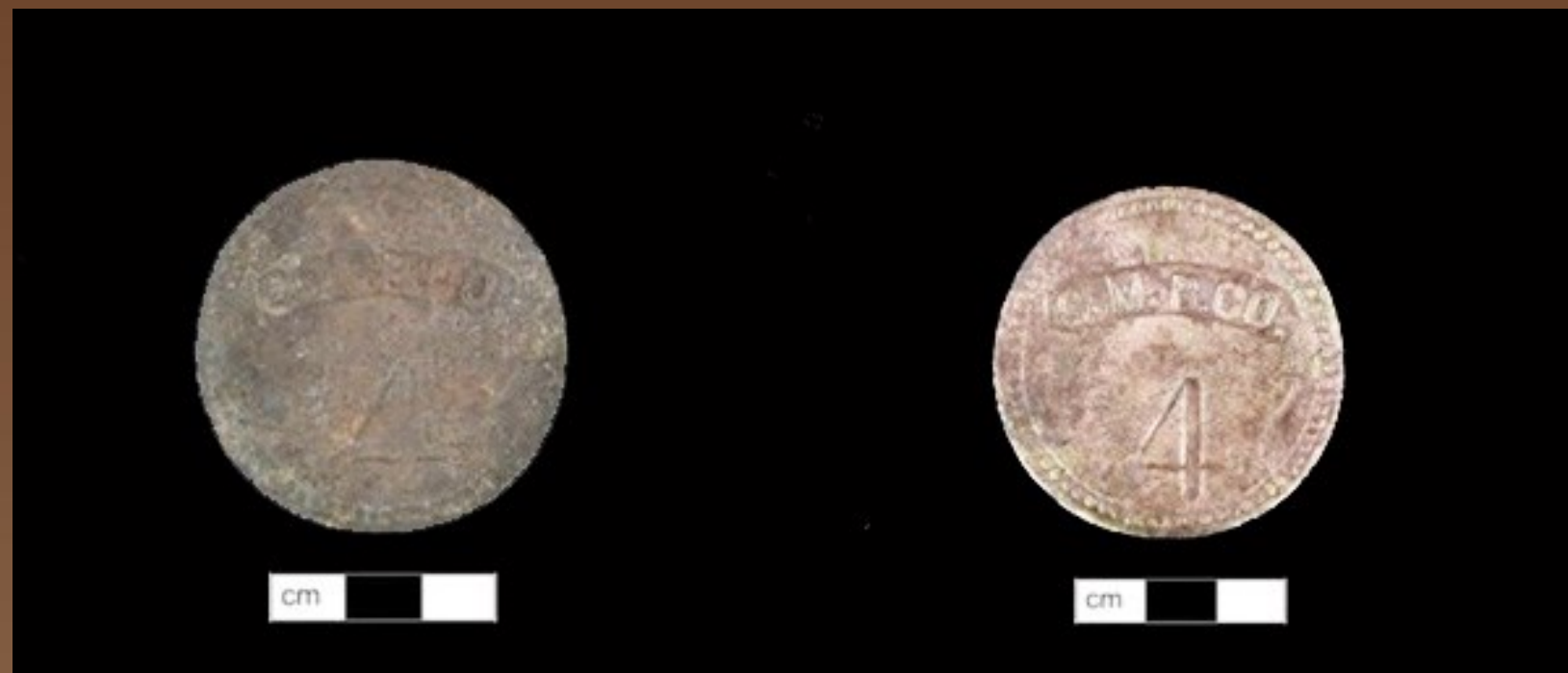
Figure A (left): Token before conservation treatment with the stamped decoration covered with corrosion. Figure B (right): Token after treatment with the stamped initials, number four, and edge decoration visible.
